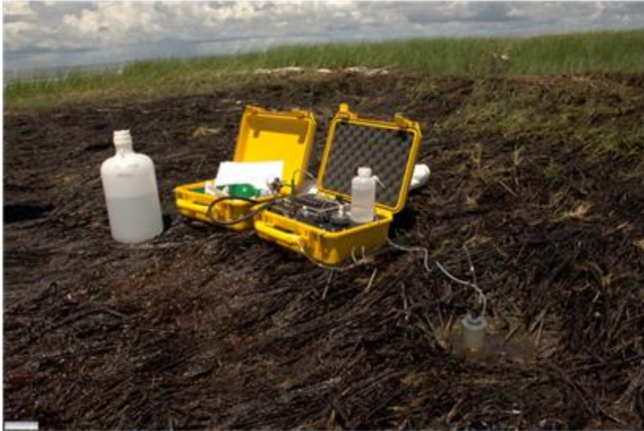
A Cohesive Strength Meter (CSM) test ion a heavily oiled marsh soil.
