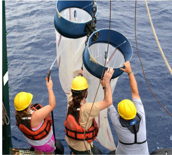
► Graduate students using bongo nets to collect plankton in the Gulf of Mexico aboard the R/V *Weatherbird II*.
