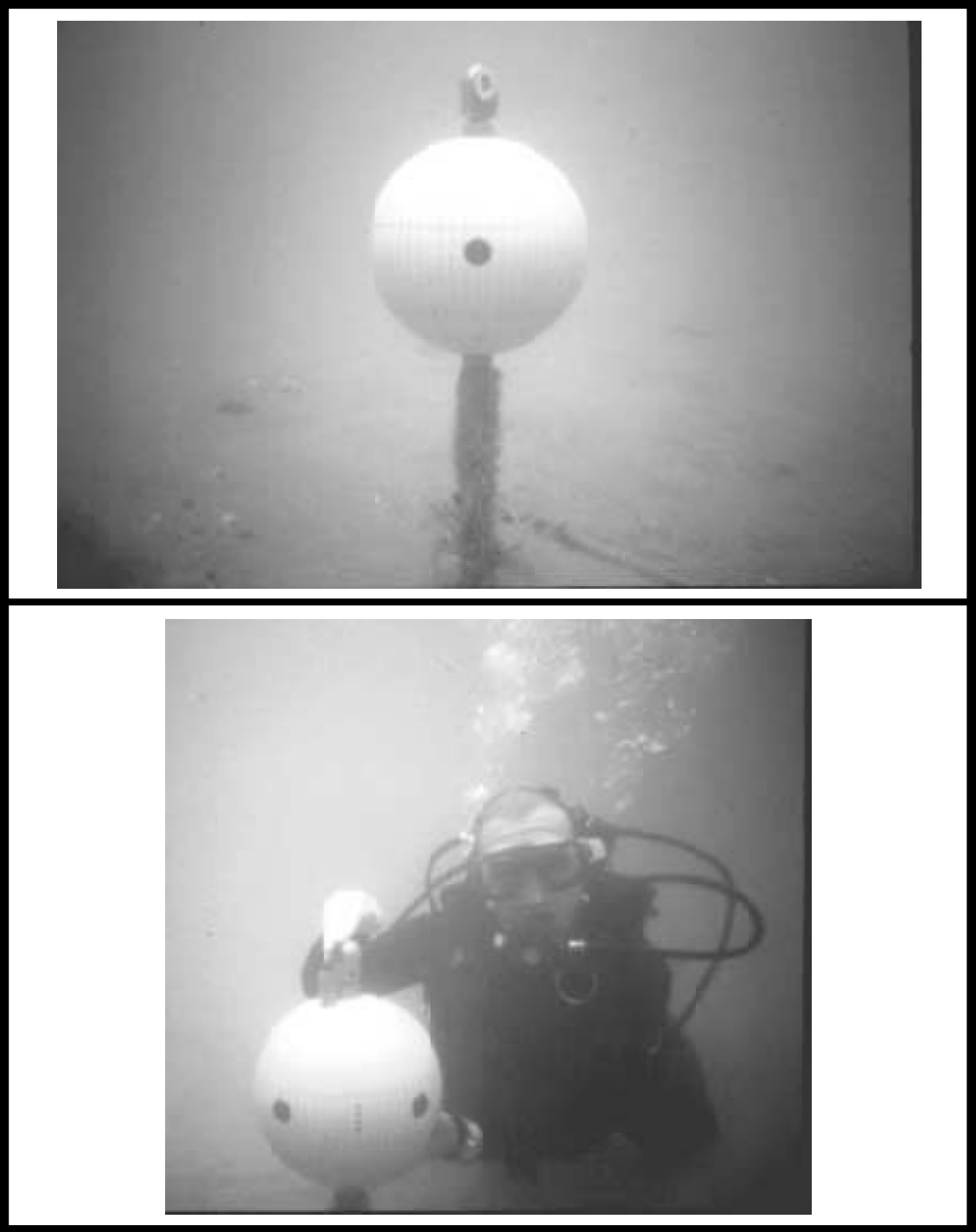
Figure 12. InterOcean S4 ® current meter deployed in both the MS and IRB study areas.
