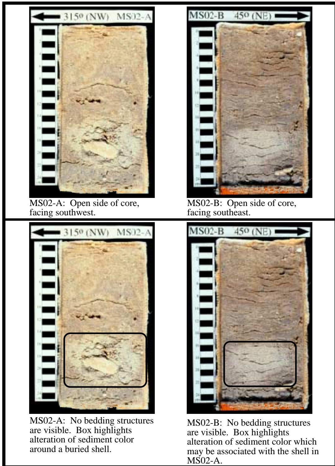
Figure 41. Embedded box core peels from site MS02 (see Figure 14 for location). Top: scans of core peels. Bottom: identification of features in each peel.
