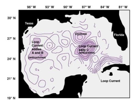
A contour map of the gulf depicts the variations in sea-surface height caused by Loop Current eddies. This map shows the Loop Current soon after it shed Eddy C in mid-September 1996. Dark purple areas indicate anticyclonic Loop Current eddies A, B, and C moving through the gulf. (Data courtesy of **George Born** and Robert Leben, Colorado Center for Astrodynamics Research).
