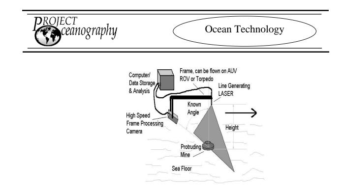
The figure above shows range scanning with a low power laser and a high speed CCD camera. Data are stored in line scan form, 256 bytes at a time in the host computer. Initial processing of "brightest pixel" information, using a threshold process, as well as the option of more sophisticated processing (successive approximation) is performed in the camera itself.
