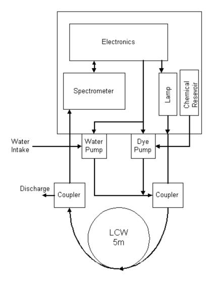
The water enters the water pump and is mixed with a dye that will determine the presence or absence of the chemical of interest. The mixed fluid is sent through the LCW, and is ejected.
