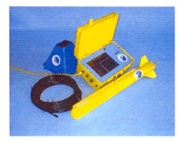
The side scan sonar plots the ship's position, the position of the object, and tracks swath coverage. The operator of the side scan sonar is able to see the big picture and is also able to zoom in on objects of interest. Below is a side scan sonar picture of a body at the bottom of a lake.
