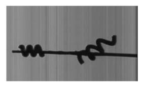
Image of a 1.5mm diameter light bulb filament and a 250 micron optical fiber at the center of the sampling tube, moving at 0.25 m/sec through the light sheet. The camera scan rate is 6000 lines/sec. The figure shows a 3.62 mm portion of the 100 mm sample cross section.
