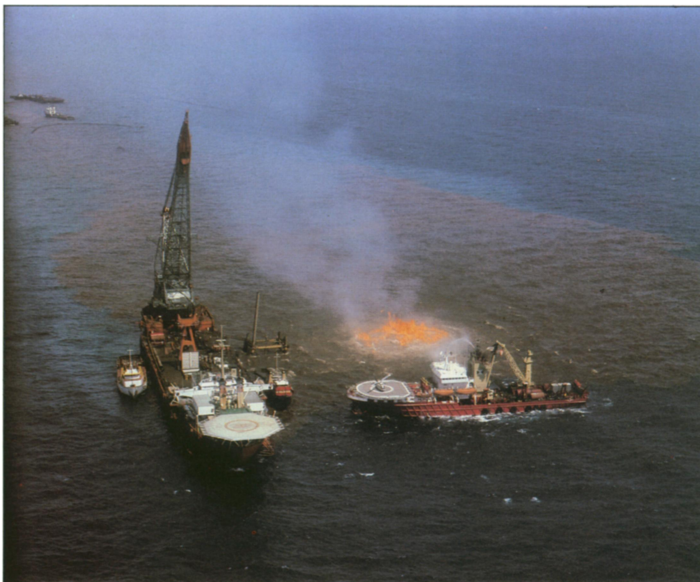
Figures 2a and b. The blowout as seen from a helicopter. Wind and current carried the oil in a north westerly direction. The rig in the foreground (left above) is a relief drilling platform. 2b on opposite page is a close-up of 2a. All photos: Olof Lindén.
