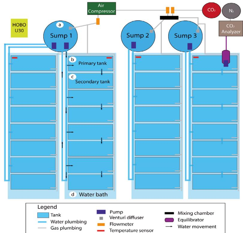
Fig. 1. Detailed schematic of ocean acidification experimental system. Letters represent the flow-through trajectory of water from the sump (a) to the water bath (d)
